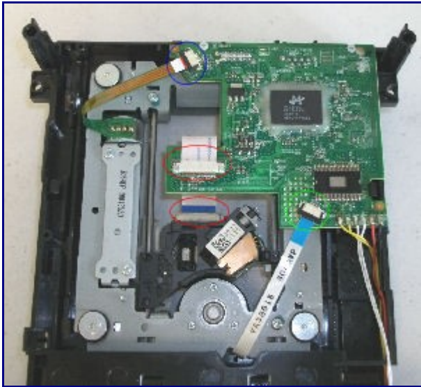
Step 18. Flip the drive over and make sure no ribbon cables have slipped out.
