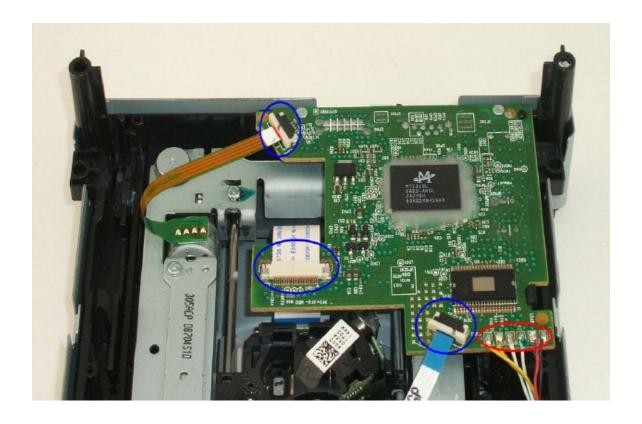
The wires circled in blue simply plug out. The wires circled in red (6 wires on DG-16D2S drive) must be de-soldered to remove the old board. The new board must be removed from the new drive (using the same method). The old board must then be soldered into the new drive. You do not need any solder to perform this task. You can use the solder that was left on the board when you removed the wires.
